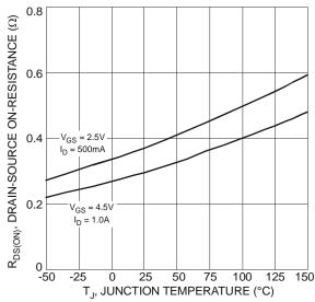
Fig. 6 On-Resistance Variation with Temperature
